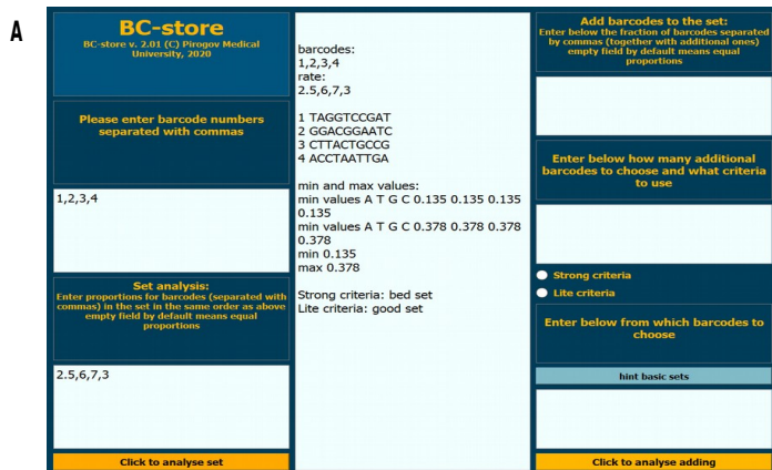
Figure 2. Layout of the desktop version with numbering of input fields and buttons. 1 – enter the current set, 2 – enter set proportions, 3 – set analysis button, 4 – output field, 5 – input proportions of the current set with the new barcodes, 6 – enter the number of new barcodes, 7 – select criteria, 8 – tip for base sets, 9 – input the barcode to choose from, 10 – start analysis of set selection.
